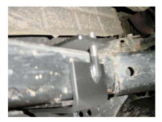
Torque to 60 ft lbs. By tightening the top bolt it will bring the Dropkick up towards the body. To move it away from the body Tighten the lower bolt.
