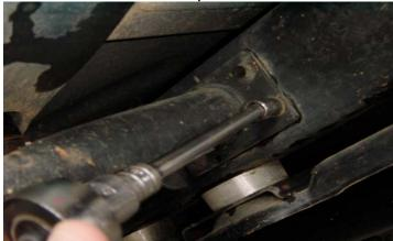
PASSENGER SIDE: Slide the Dropkick onto the frame using the C channel to hold it to the frame. The end of the dropkick with the longer leg goes on the forward side of the Dropkick.
