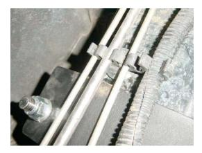
As you did on the passenger side torque the locknuts to 45 ft lbs.
