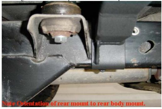
Install the backing plate over the Dropkicks studs matching the orientation of the outside bracket. Install the lock washer first followed by the 5/8 locknut.
