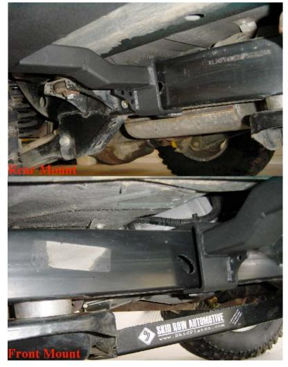
Position the rear bracket against the rearmost body mount as shown in the picture:
